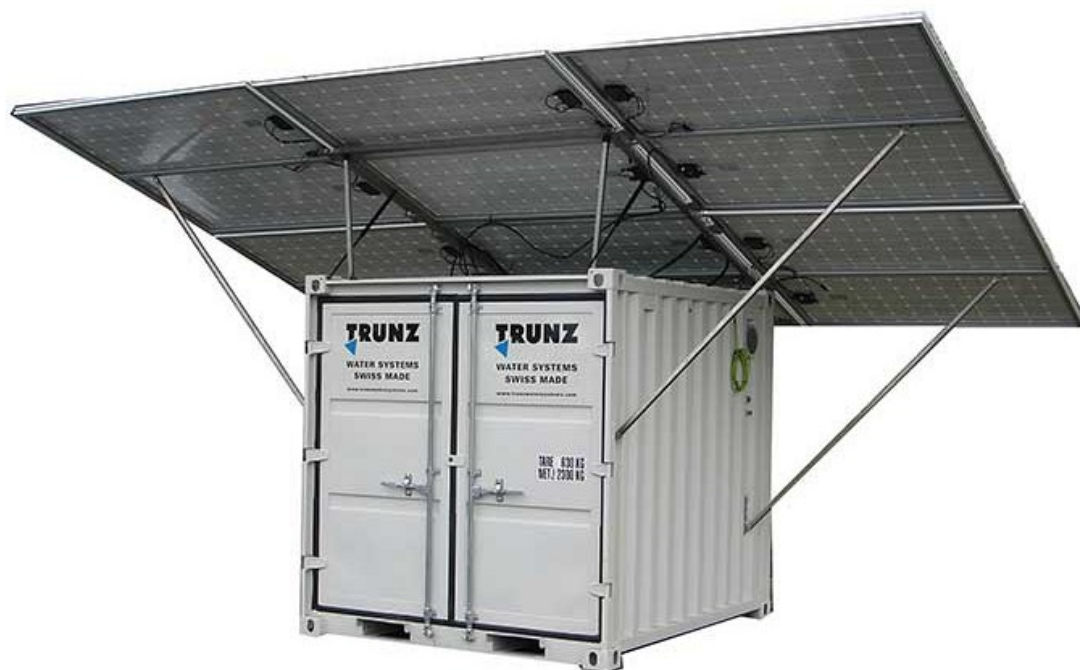
Figure 10 – Solar powered containerised system for brackish water (up to 18,000 ppm salt content) and seawater desalination (up to 42,000 ppm salt content). A system has been installed in a remote agriculture farm, near Al-Alin Desert, United Arab Emirates. (Source: https://www.trunzwatersystems.com/index.php )
